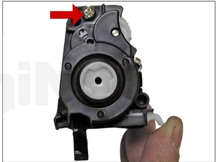
24. Install the gear end cap and screw.
