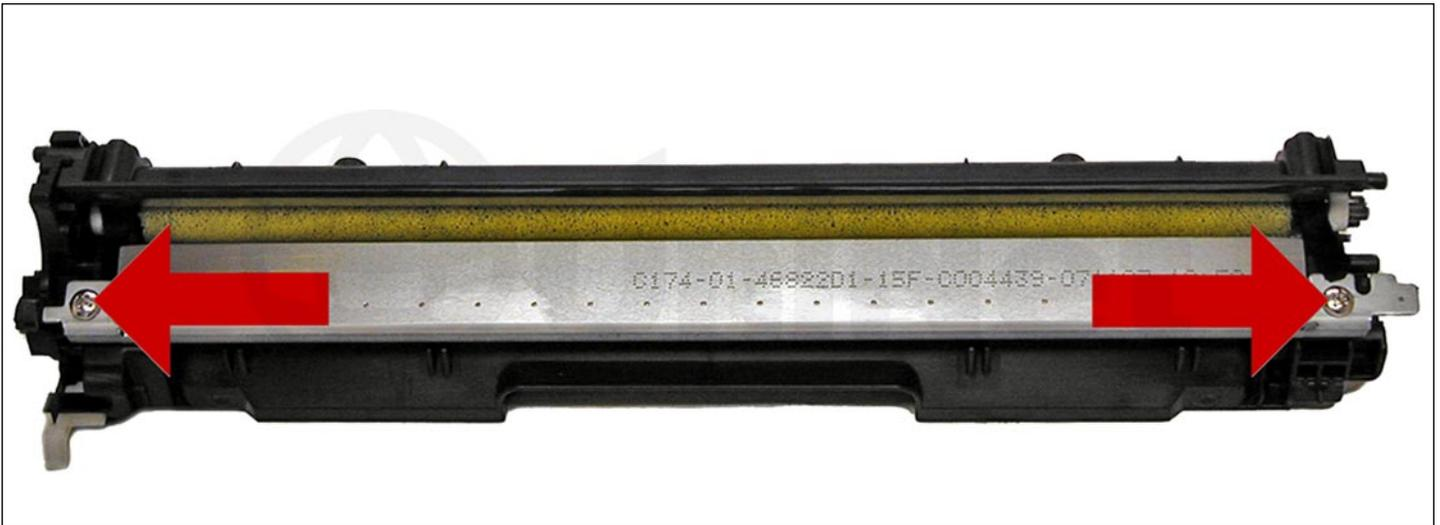
13. Remove the two screws and doctor blade.
