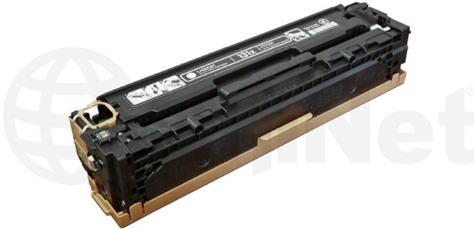
First released in August 2012, the HP LaserJet Pro 200 M251/M276 (131 Series) color laser printers are based on a 14-ppm black, 14-ppm color, 600-DPI engine. The 131 series of cartridges are an all-in-one type that consists of the toner supply, drum, and waste chamber. These machines use an in-line, or single-pass system. It's basically a rectangular-shaped cartridge that comes with a toner seal and a snap-on drum cover across the bottom to protect the drum (see photo above).
