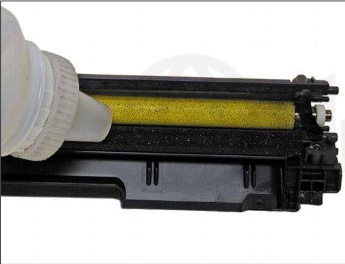
15. At this point, while tight, you can clean and fill the hopper with toner for use in the HP 131 Series.
