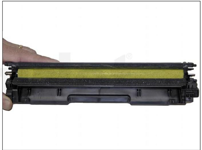
16. If you have not already done so, fill the hopper with new replacement toner for use in the HP 131 series, and install the feed roller.
