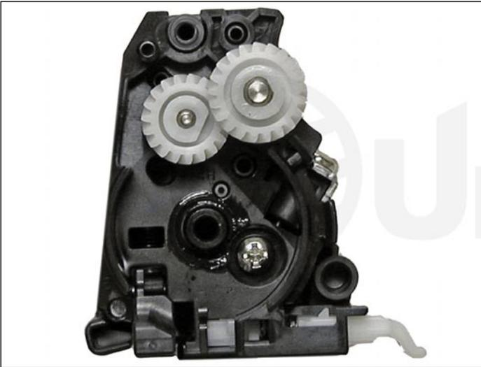
23. Replace the two gears on the feed and developer roller shafts.
