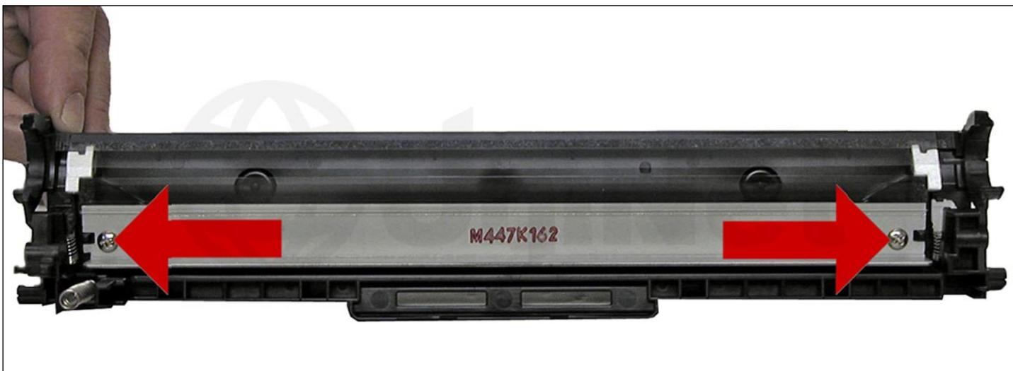
5. Remove the two screws and wiper blade shown.
