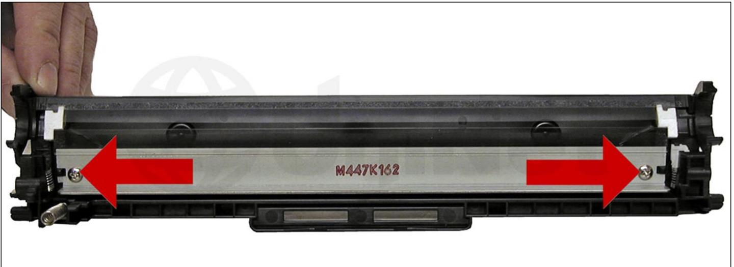
7. Coat the new wiper blade with your preferred lubricant and install.
