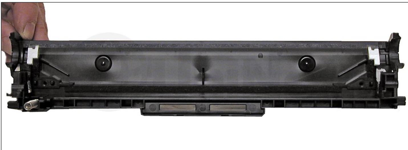
Wiper blade and screws removed.
