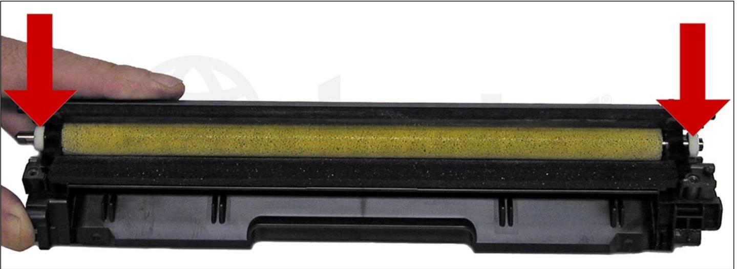
The opposite side bushing is integral to the hopper. If you wish to install a seal, change the feed roller, or just have better access to the hopper, the feed roller must be pulled over to one side compressing the foam. First remove the two white felt seals.
