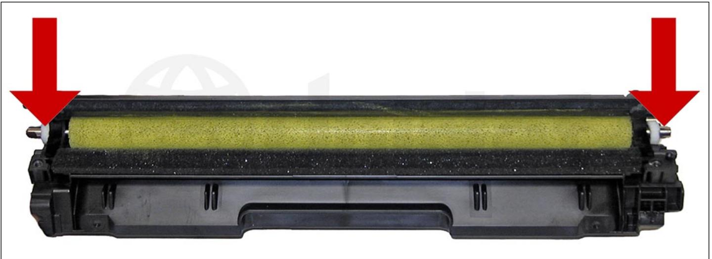
17. Install the two white felt seals on the feed roller shaft.
