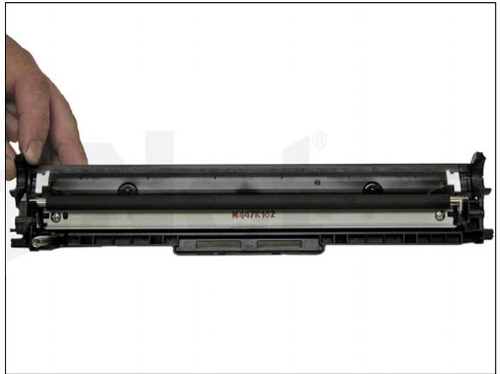
8. Install the cleaned PCR.
