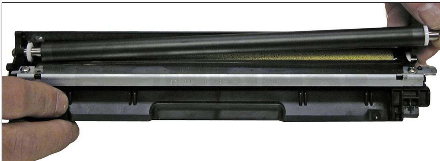
12. Slide the developer roller over and remove.
