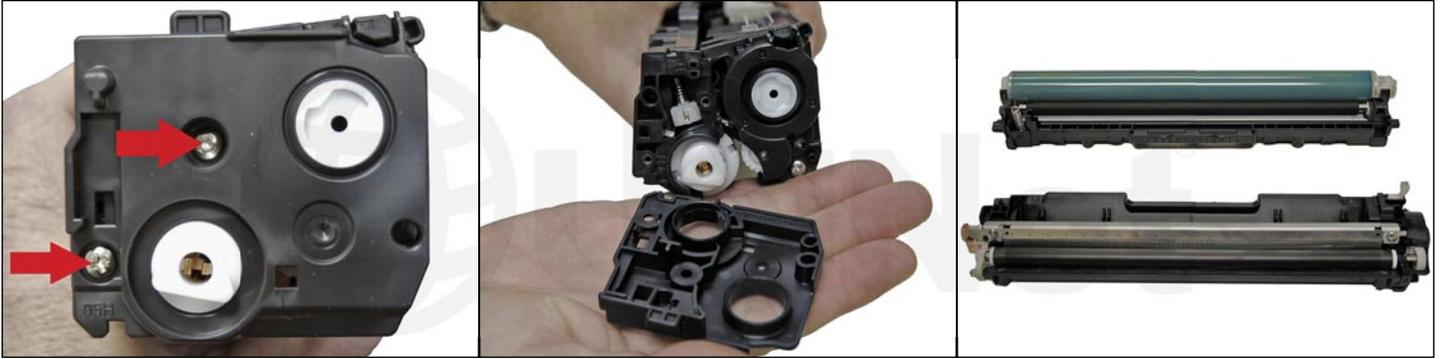
2. On the right side, remove the two screws and end cap.
