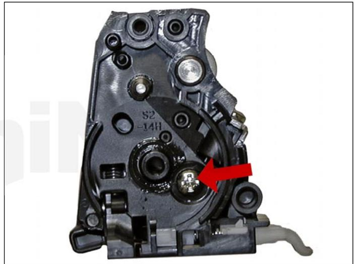
20. Install the inner end cap and screw.
