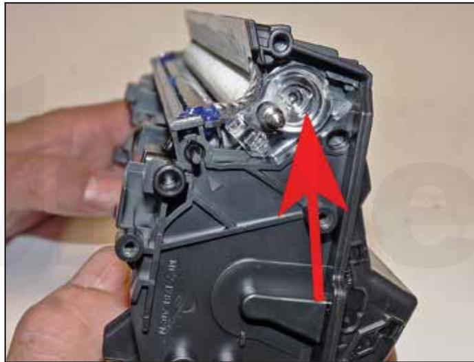
24. The clear bushing that holds the feed roller in place in previous style cartridges were removable, but in this series it is glued in place. The only way to clean and fill the supply chamber is to melt a hole in the chamber at this time.
