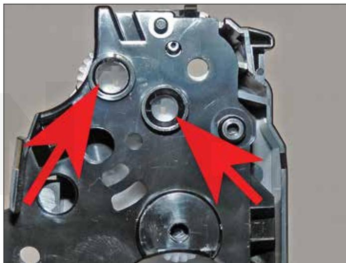
33. Set the gears inside the end cap so that the two drive gears for these shafts have their flat side also on top.
