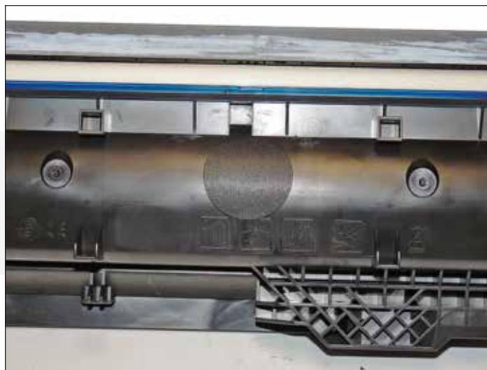
27. Place a sealing label over the hole to seal it off.
