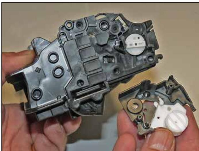
19. On the contact side, remove the two screws. Remove the small top end cap with the white gears.
