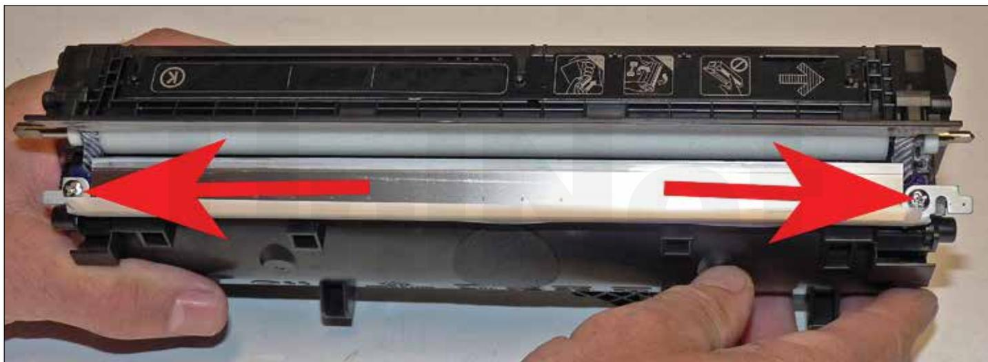
29. Use the appropriate shims to set the gap. Install the doctor blade and two screws.
