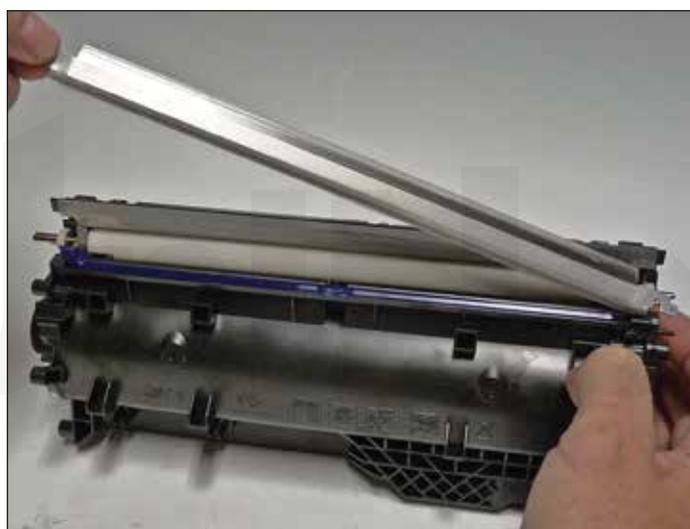
22. Remove the two screws from the doctor blade. **IMPORTANT:** The **Right** (gear side) screw uses a **LEFT-HAND THREAD!** Lift the blade up and twist so that it comes free from the cartridge. **KEEP THE LEFT-HAND THREADED SCREW SEPARATE!**
