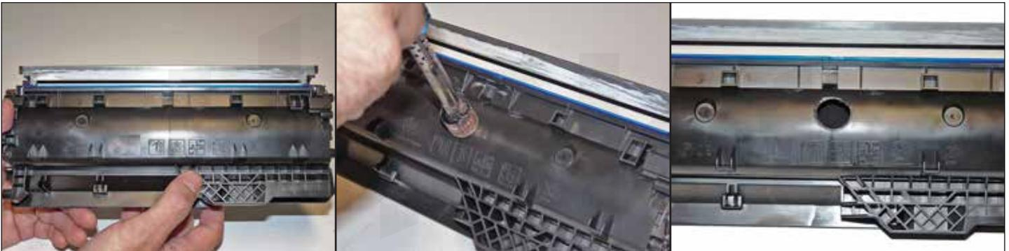
**NOTE:** These cartridges have a self-removing seal that is not accessible from the outside of the hopper. To install a seal it looks like the hopper will have to be split. Testing is ongoing for this possibility.
