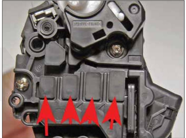
Note that there are no metal contacts on this end cap as you would normally see. The contacts are there, but are now made of conductive plastic.
