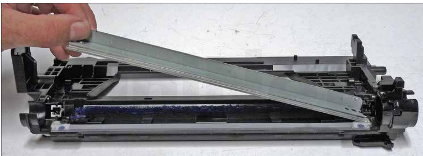
9. Remove the two screws from the wiper blade.
