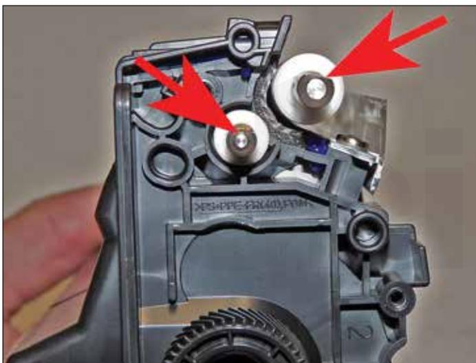
32. Set the developer roller shaft and feed roller shafts as shown. Flat side up.
