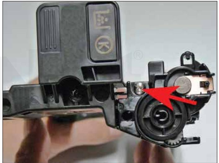
15. Clean and replace the conductive grease on the drum axle. Install the end cap and screw.
