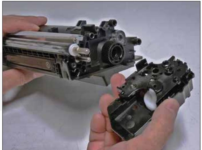
18. Remove the inner and outer end cap together as one piece. Note that the gears stay in the end cap!
