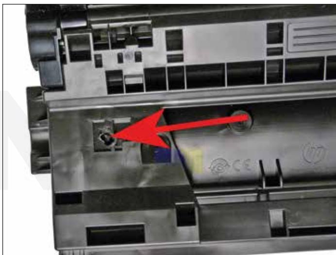
3. Drill a small hole in the top of each side of the cartridge as shown.
