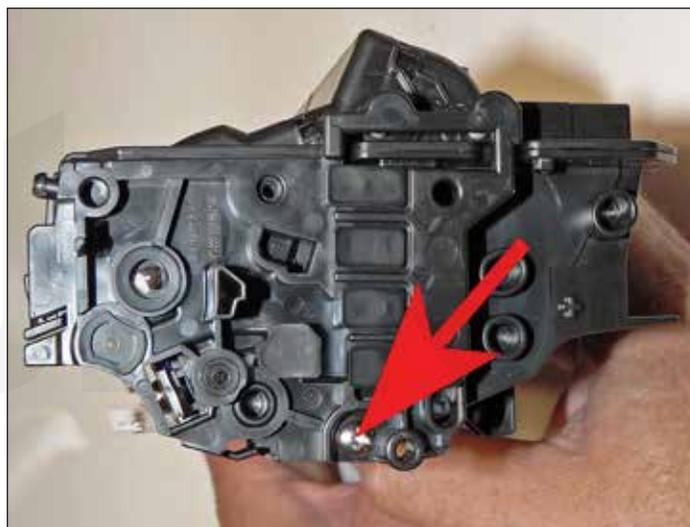
30. Install the inner contact end cap and screw.
