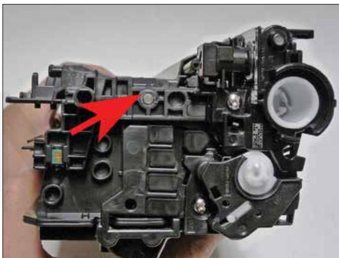
2. With a razor knife, carefully shave the plastic from the heads of the hinge pins on both sides of the cartridge.
