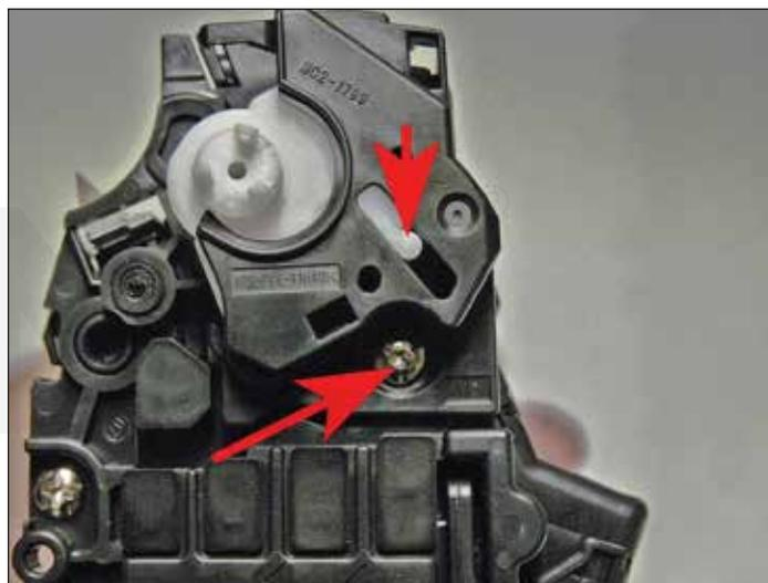
35. Place the base of the triple gear on the developer roller shaft and fit into the spring assembly on the small end cap.
