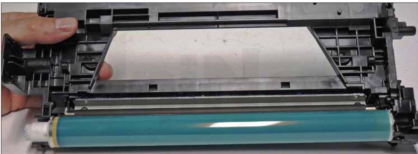
14. Install the drum long hub side onto the remaining end cap.
