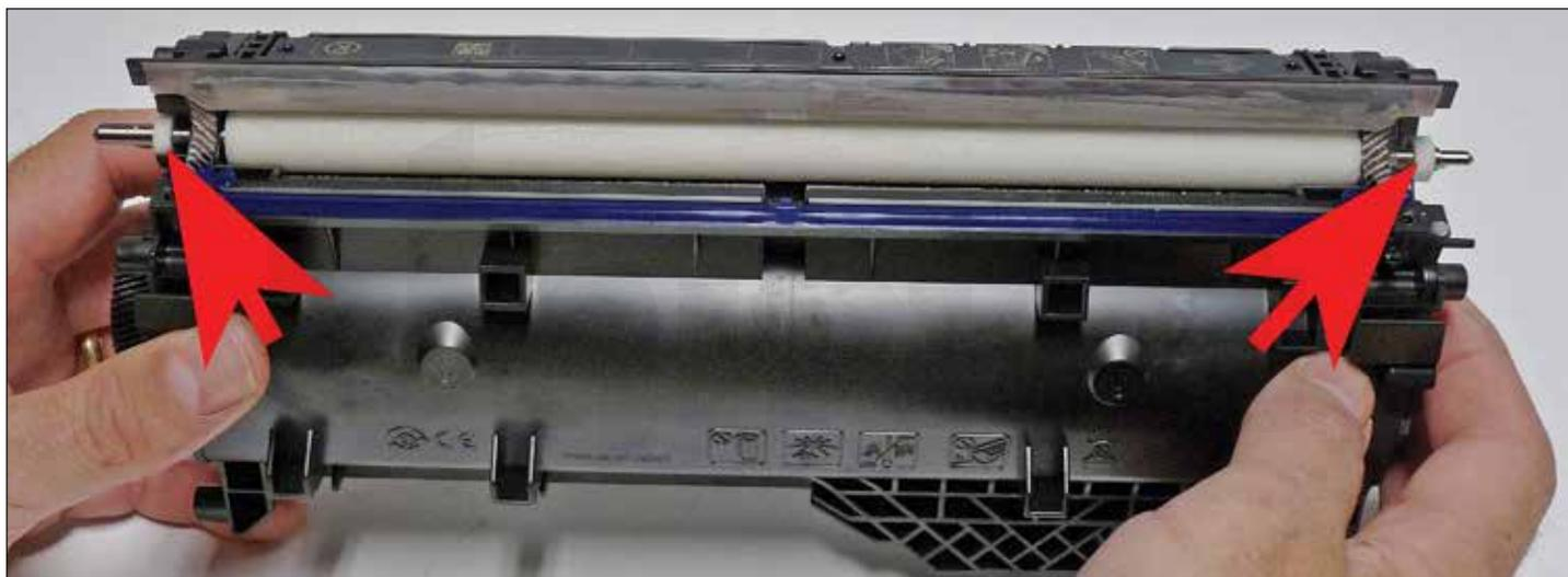
23. Remove the round white felt washers from both sides of the feed roller to prevent them from being lost.
