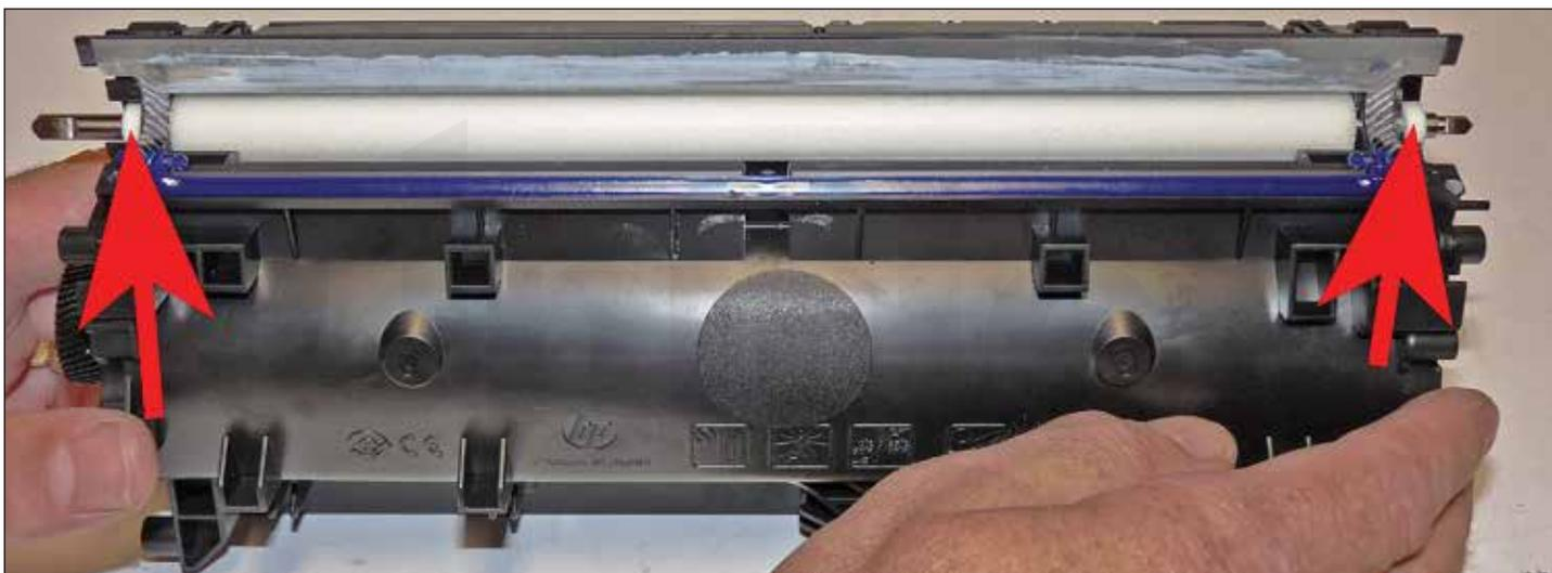
28. Install the feed roller felt washers.
