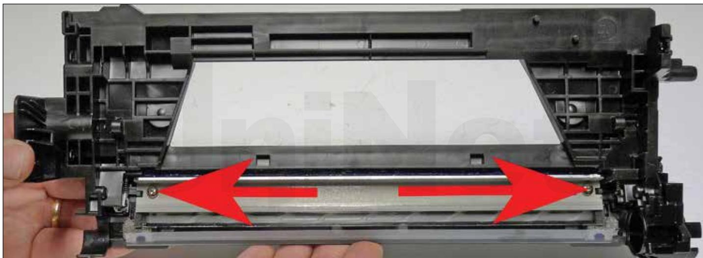
12. Install a new or cleaned, lubricated wiper blade and two screws.
