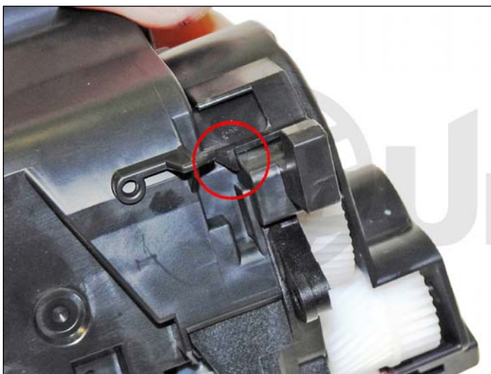
22. Press in on the tab and remove the end cap.
