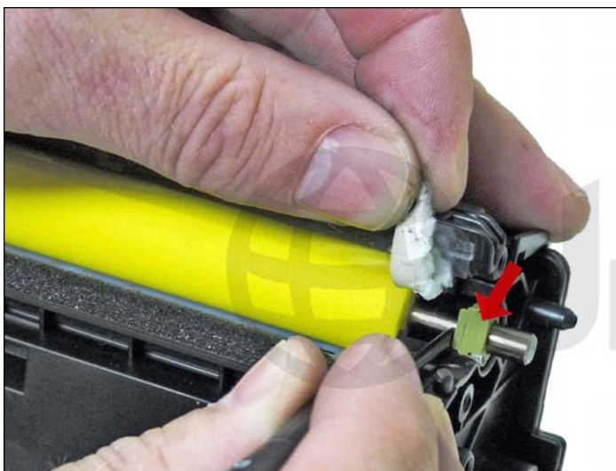
31. Pry out the feed roller bushing from the right side.
