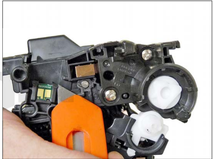
50. Remove the chip by cutting the plastic off the edges of both side of the chip.
