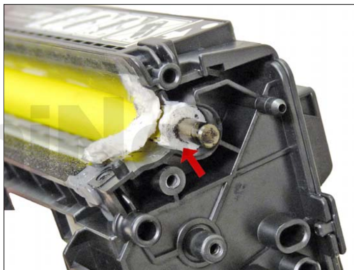
30. Remove the white felt washers from both sides of the developer roller.
