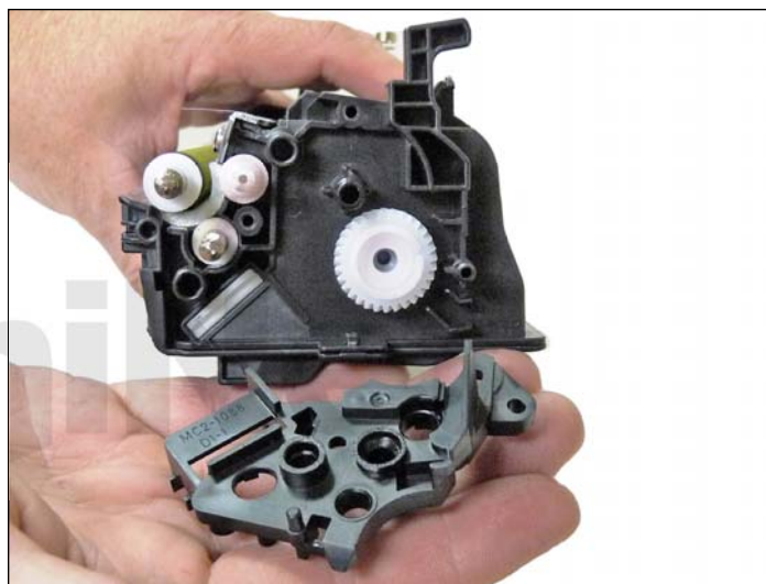
24. Remove the two inner screws and inner gear end cap.
