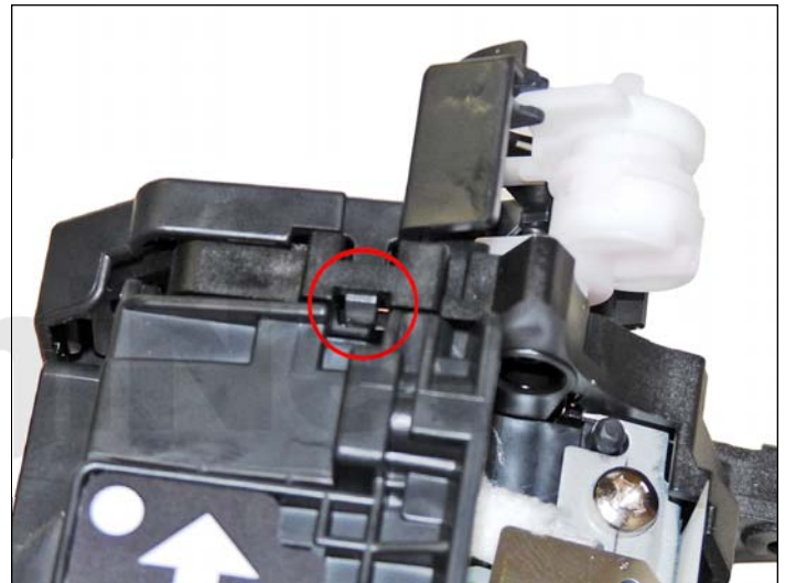
26. On the opposite side end cap remove the single screw and press in on the tab to release it.
