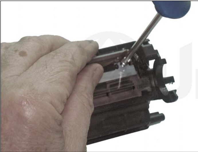
5. Remove both screws below the transparent sealing blade, and take the wiper blade out.
