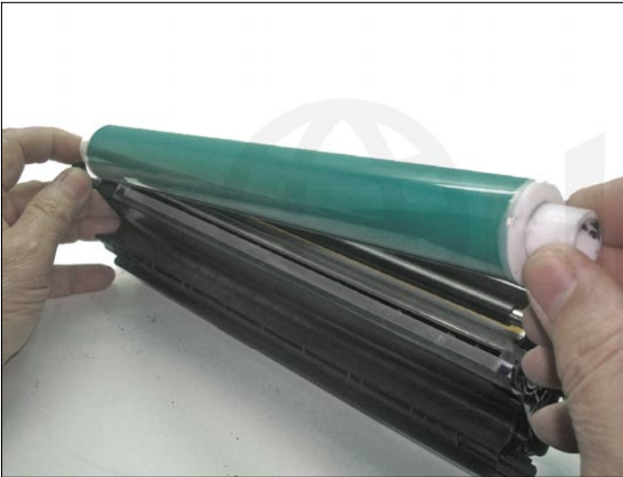
3. Carefully remove the OPC drum.
