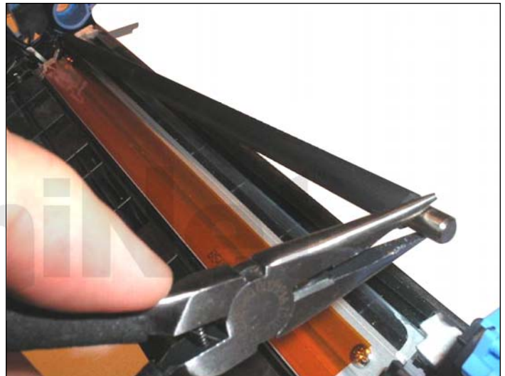
19. Using a pair of needle nose pliers, gently lift up the PCR from one side.
