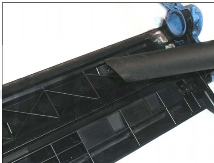
26. Use a vacuum to clean out the waste bin of used toner. This will allow you to re-use the OEM adhesive strip to reassemble the wiper blade. NOTE: Do not use compressed air, as it will only scatter the used toner and coat the adhesive strip, rendering it useless.
