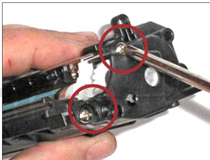
43. Remove the two screws from the non-contact (gear-side) end-plate shown. Carefully remove this plate to access the gears inside.
