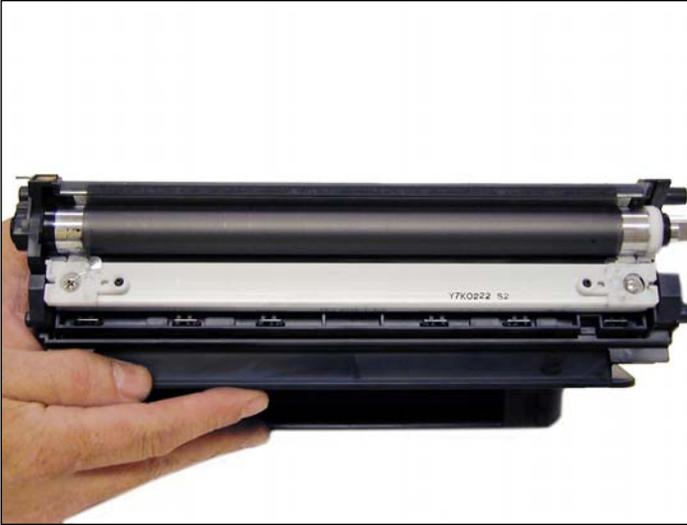
33. Install the MRS assembly. Make sure the clear strips from the DB ride on top of the magnetic roller.
