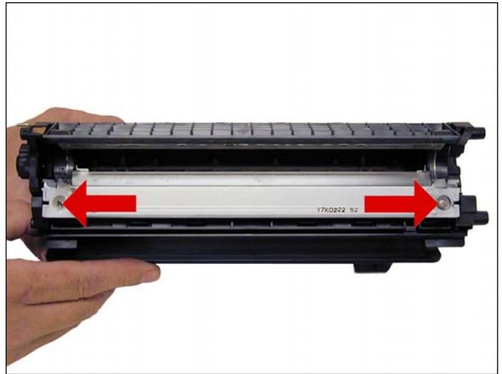
31. The upper mag. roller section of the toner hopper is different in that it "floats" on a series of foam seals. The upper half can be removed from the hopper, but some of the seals will be destroyed. This may become necessary in order to seal the cartridge we will keep you informed as our testing continues. The foam isolates the mag roller from the vibrations of the mixing augers, and allows smoother prints.
