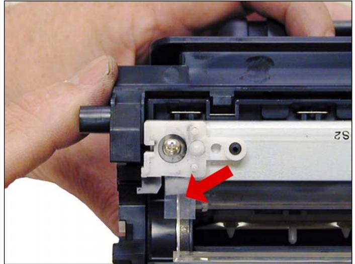
25. Remove the two doctor blade screws and the doctor blade. Note the clear plastic strip that covers the DB screws. Slide the screwdriver under the strip. Be careful not to damage the strip!
