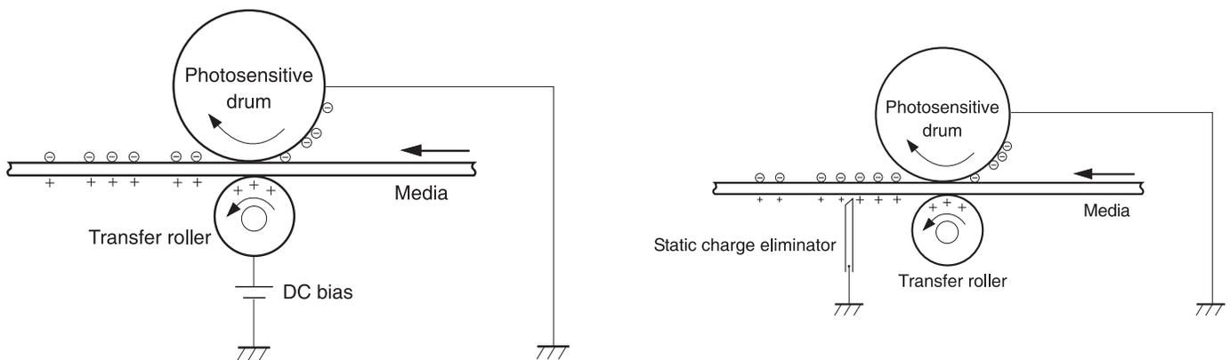
In the **fourth** step (transfer block) the toner image is then transferred to the paper as it passes below the drum by the transfer charge roller, which places a positive charge on the back of the paper. This positive charge causes the negatively charged toner on the drum's surface to be attracted to the page. The small diameter of the drum, combined with the stiffness of the paper causes the paper to peel away from the drum.
