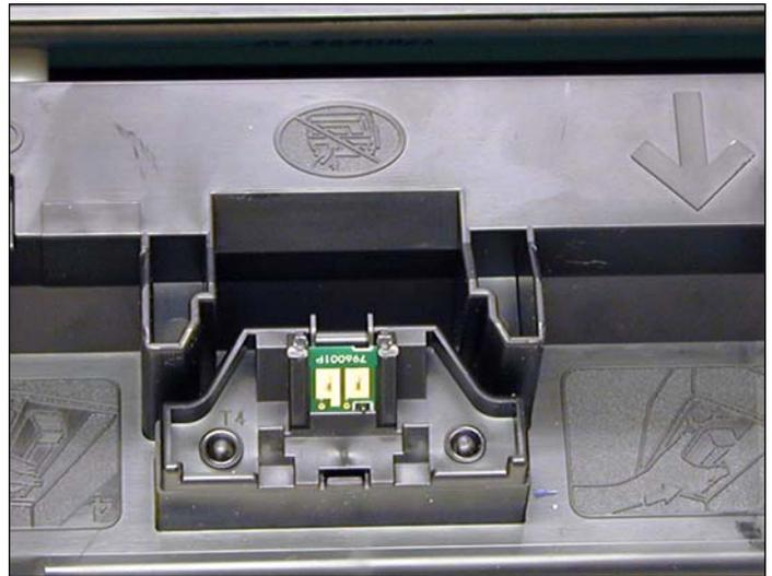
45. Remove the old chip from the top of the cartridge by slicing the melted plastic off with a sharp X-Acto knife. Replace the chip, then lock in place with a small dab of glue from a hot glue gun. Replacing this chip will enable the toner low functions of both the cartridge and the machine again.
