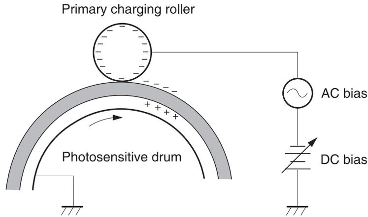
In the **first** step, the Primary Charge roller (PCR) places a uniform negative DC Bias voltage on the OPC drum surface. The amount of the negative DC Bias placed on the drum is controlled by the printer's intensity setting. This process is part of the latent Image formation block.
