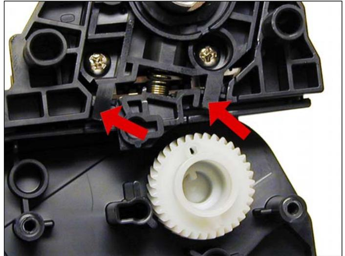
35. Install the holder 2 screws and spring. Make sure the screw holes line up, and that the two locking tabs on the bottom of the holder are in the correct place.
