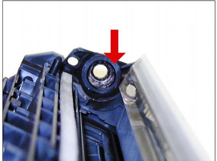
29. There are HP-4000 style magnetic roller bushings on each side of the roller. While these are holding up well in our initial tests, this may be an area where wear will cause banding. One will stay in the hopper, and one comes off with the mag. Roller assembly.
