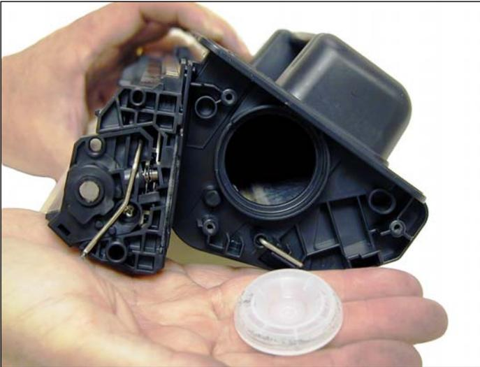
26. Remove the fill plug and clean out all the remaining toner in the supply hopper
