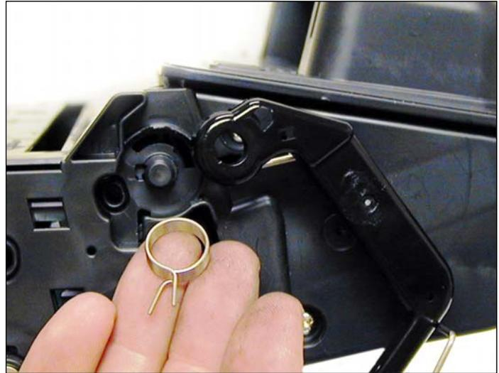
3. On the opposite side of the cartridge, carefully pry off the drum cover plastic arm. The spring will probably pop off, take care not to loose it. We will go over the installation at the end of this article. Remove the drum cover assembly.
