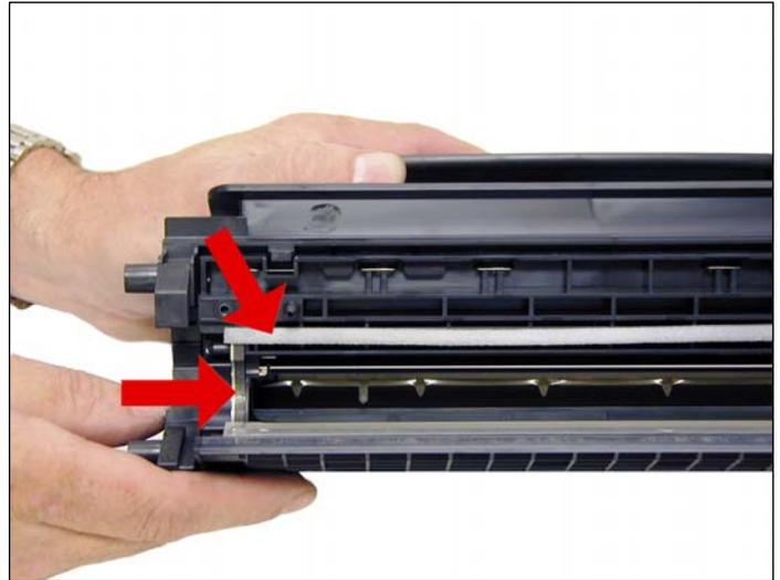
27. Note the magnetic seals on the MRS and the DB sealing foam. Make sure both are clean.
