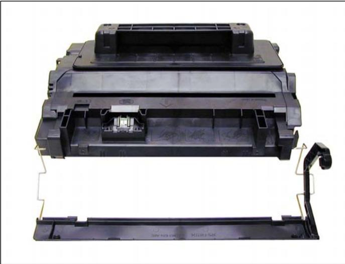
4. Remove the metal bar from the left side, and remove the entire drum cover assembly. Make sure you put the spring in a safe place.
