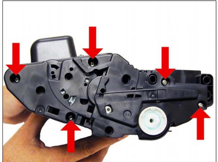
5. Remove the five screws on the right side end cap.
