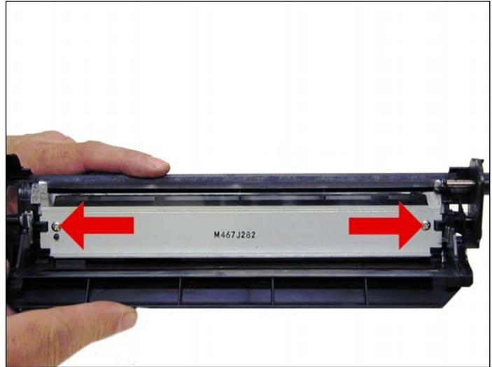
15. Install the new wiper blade and two screws.
