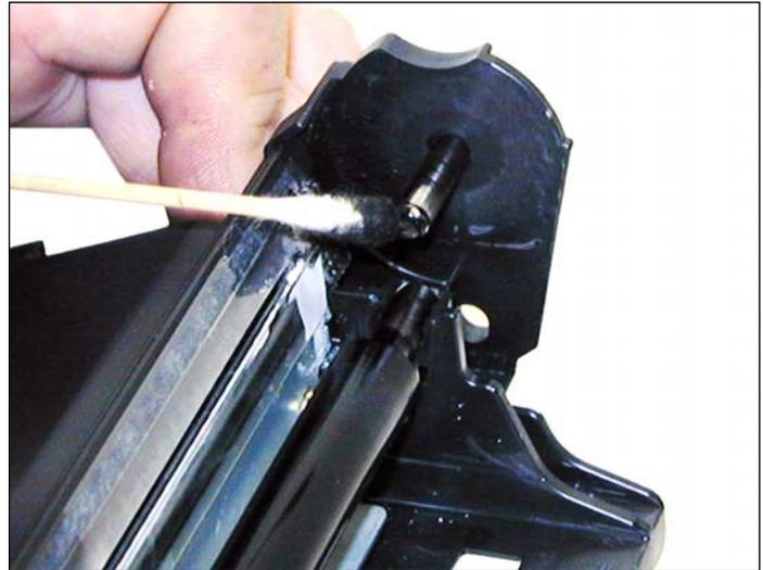
18. On the drum axle pin, clean off the old conductive grease and replace with new.
