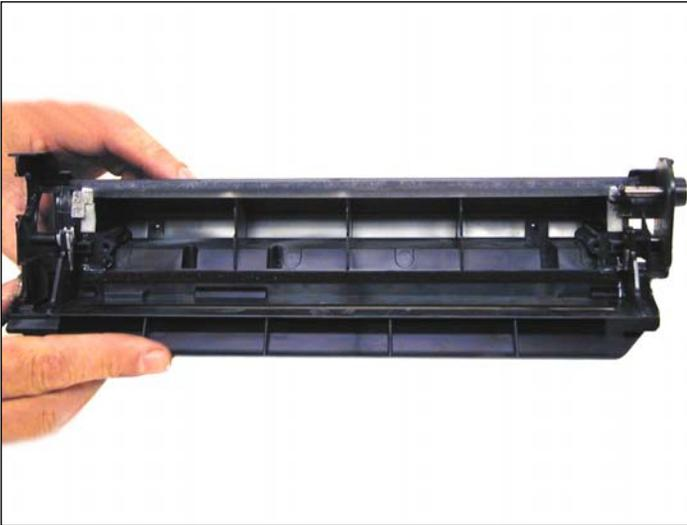
14. Due to the high speed and page counts of these cartridges, we recommend that the wiper blades be replaced. Make sure that the wiper blade foam seals are clean.
