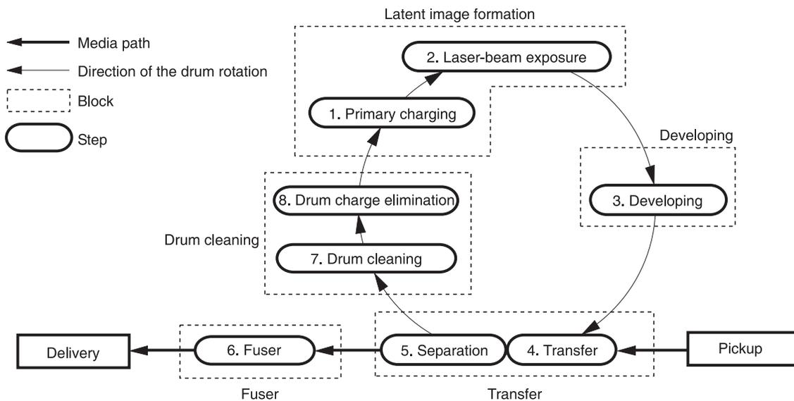
The image formation process consists of 8 steps which are split up into five functional blocks.
