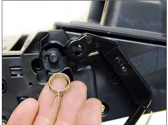
3. On the opposite side of the cartridge, carefully pry off the drum cover plastic arm. The spring will probably pop off, take care not to lose it. We will go over the installation at the end of this article. Remove the drum cover assembly.
