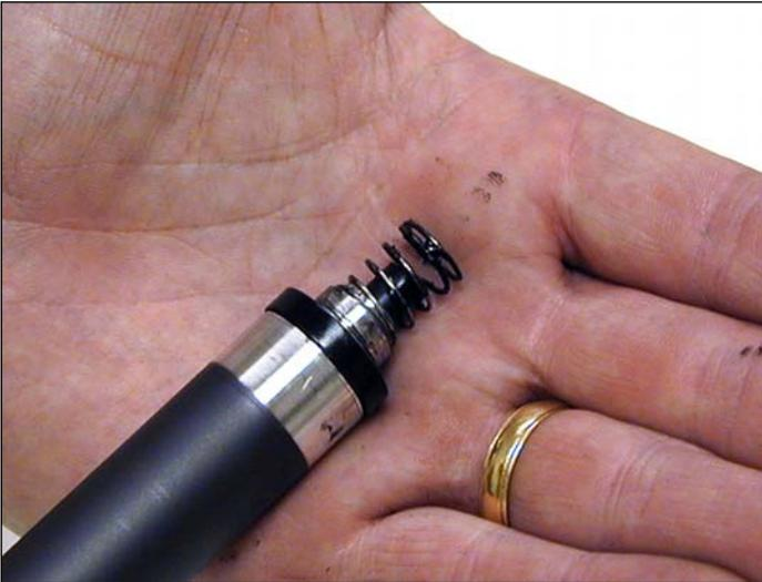
28. Note also the new heavy duty style magnetic roller contact. This when combined with the new larger diameter of the roller, allow the cartridge to run at the higher speeds that these machines are capable of.
