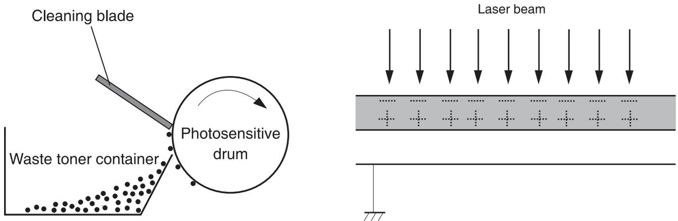
In the **seventh** step (Drum cleaning block) the OPC drum is cleaned. On average, approximately 95% of the toner is transferred to the paper during the print cycle. As the drum rotates during printing, the remaining 5% of the toner that is on the OPC drum is cleaned off the drum by the wiper blade. It is then guided into the waste chamber by the recovery blade, and stored in the waste chamber.
