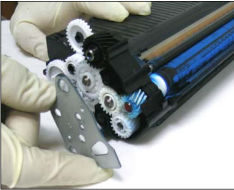
13. Remove the end plate.
