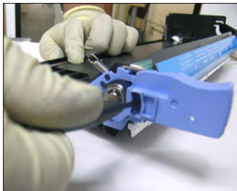
40. To disassemble the drum unit, first remove the two screws on the blue cartridge installation handle on the gearless side as shown.
