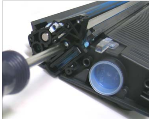
21. Now remove the roller support plate by removing the two screws as shown.
