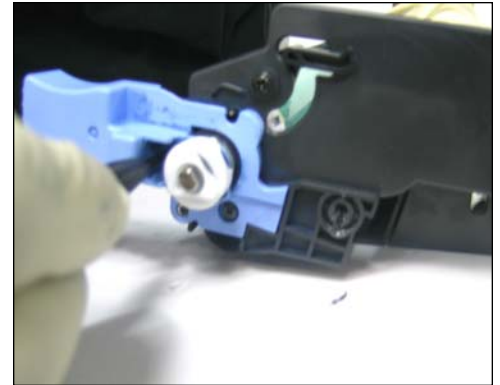
45. Remove the two screws on the cartridge installation handle at the opposite end as shown.
