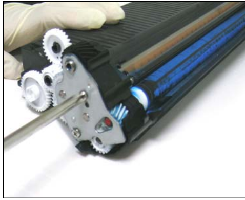
12. Remove the two screws on the end plate as shown.
