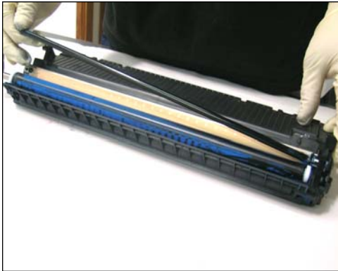
20. Once the gear side support plate is removed, the toner charging roller should be loosened for removal.
