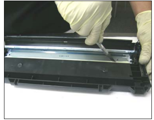
51. To remove the wiper blade, first cut through the OEM seal with a utility knife.
