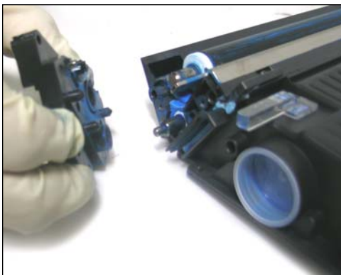
22. The roller support plate can now be removed.
