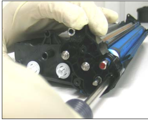
18. Remove the gear side support plate by removing the two screws as shown.
