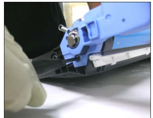
40. To disassemble the drum unit, first remove the two screws on the blue cartridge installation handle on the gearless side as shown.
