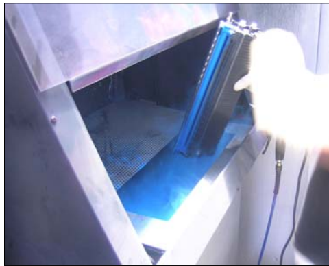
34. Empty residual toner and clean cartridge using air pressure.
