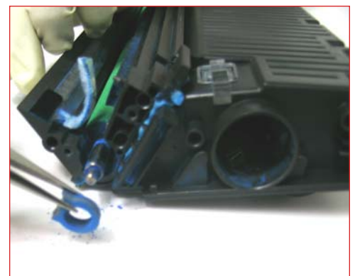
32. Remove the rubber bearing that is holding the supply roller in place.
