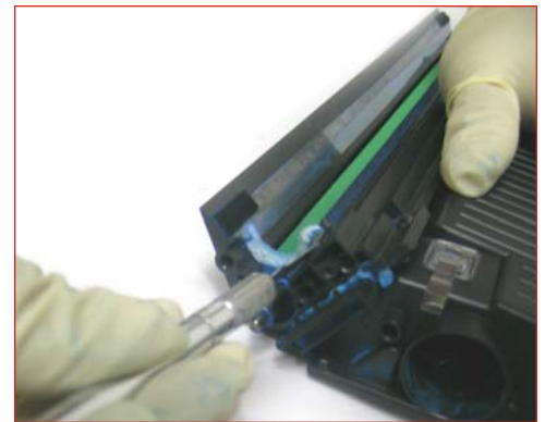
29. Use a utility knife to carefully separate the mag roller felt from the supply roller as shown in the following steps.
