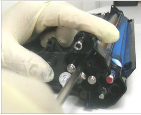
18. Remove the gear side support plate by removing the two screws as shown.
