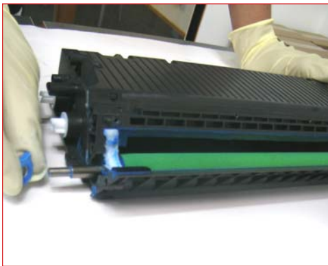
28. *REMOVING THE SUPPLY ROLLER. Remove the felt o-rings from opposite ends of the supply roller as shown.
