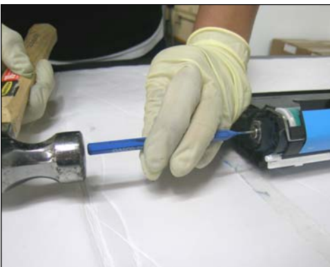
46. Use a pin puncher tool and hammer to loosen the drum axle inside. Punch in from the gearless side.
