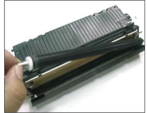
35. Then, remove the developer roller by pulling it sideways. Be careful not to lose the white bushings on each end as they can easily fall off.
