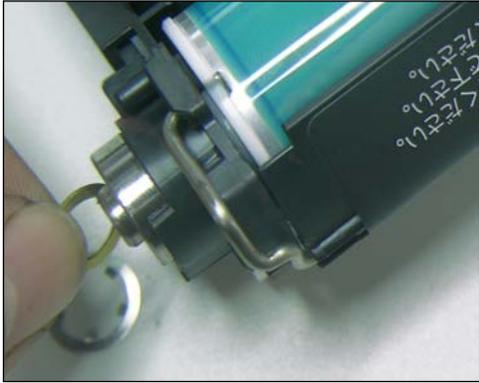
51. Apply the washer, then press the star-lock clip back over the shaft. Check that each end of the shaft is sitting in place correctly.
