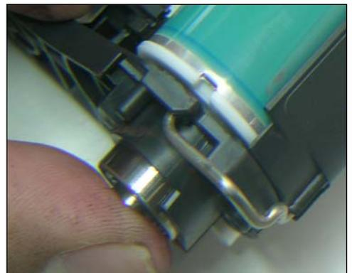
50. Hold the left-hand end bearing in place while inserting the shaft. The shaft will need to be turned slightly to engage the shaft-locking pin into the drum key slot.
