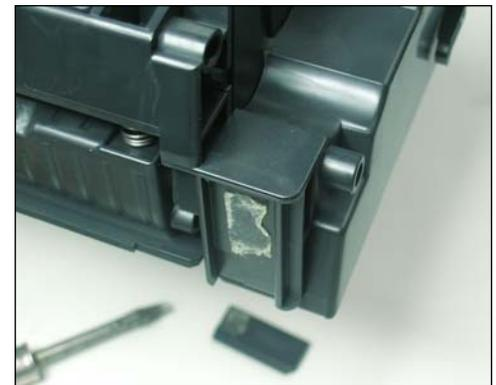
**REMOVING THE OEM CHIP**
