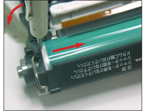
17. Wedge a flat-head screwdriver down the left side of the drum as shown. Tilt the screwdriver sideways to force the drum to the right. This will also push the shaft out the right-hand end.
