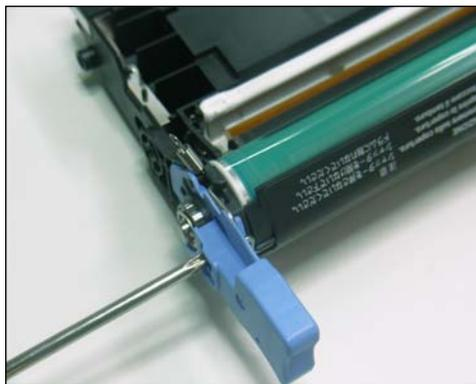
14. Using a small Phillips screwdriver, remove the screws that are located on the blue cartridge handles shown. The cartridge handle on the left-side will easily come off after removing the screw.
