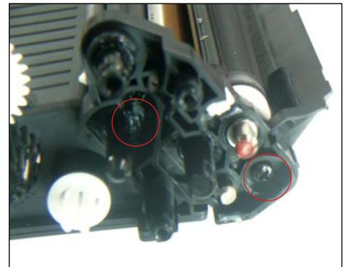
32. Gears removed. Remove the two screws that hold the roller support plate in place, then slide the plate out.
