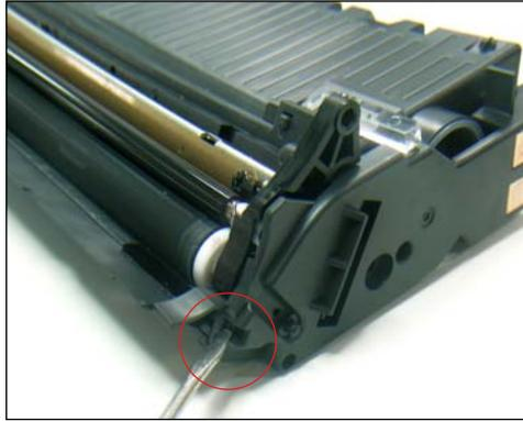
25. Use a flat-head screwdriver to press in and unclip the supporting clip in the area shown. It will be necessary to pull the cap away while pressing the clip in.
