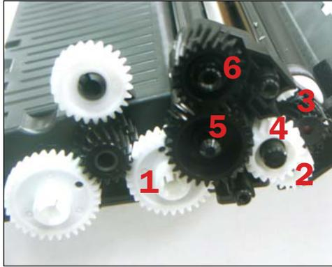
43. Install the gears in order from one to six as shown. Check that the gears are the correct way.
