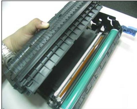
12. Lift the toner hopper portion of the cartridge away from the drum section as shown.
