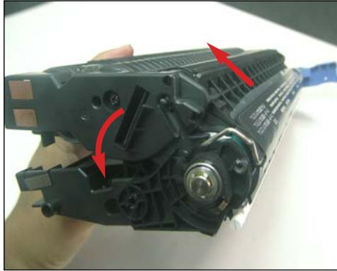
52. Assemble the two halves together. It is important to raise the drum shutter upward and lower the toner hopper downward under the shutter to prevent damaging the shutter blade.
