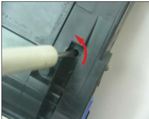
6. Insert a 3mm (1/8-inch) flat-head screwdriver with wide tip into the slot hole with the flat portion of the tip facing the pin. Push the screwdriver in behind the pin and turn in either direction. This action will push the pin out.
