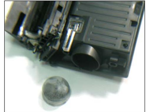
38. Using needle-nose pliers, pull out the toner fill plug. Remove residual toner and clean the hopper thoroughly using compressed air or vacuum. Fill with new toner and install the fill plug.
