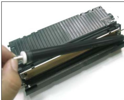
40. Install the developer roller as shown.
