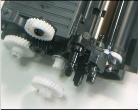
42. Install the gearside roller support plate back in place.
