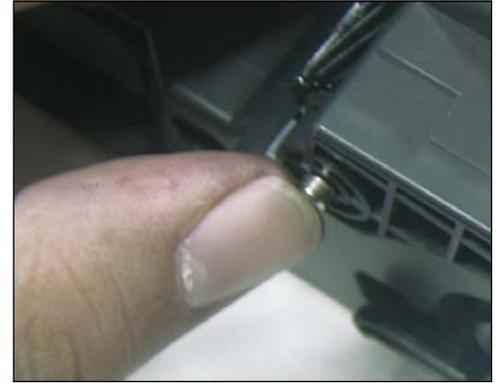
53. Insert the two cartridge pins and press fully in place.
