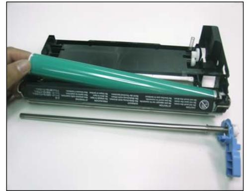
20. Carefully maneuver the left-hand end of the drum upward and lift the drum away from the cartridge as shown. If the drum is reusable, store it correctly, keeping it away from light.
