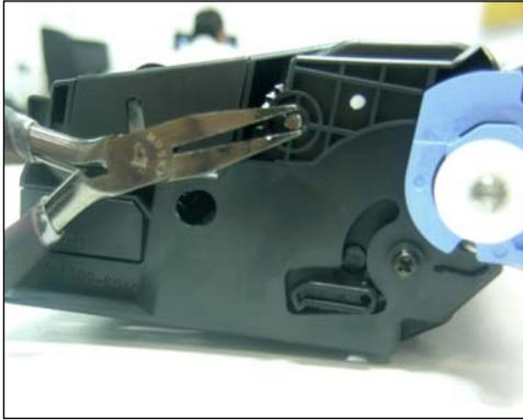
8. Grip the pin head with a pair of pliers and maneuver the pin to extract it out.
