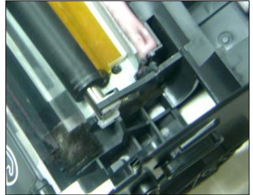
47. Install the PCR back onto the saddles shown.
