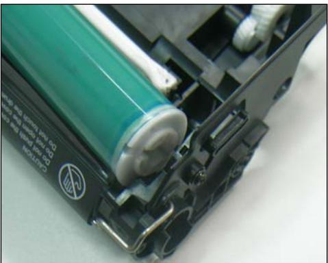
48. Insert the keyed end of the drum into the right-hand end of the cartridge.
