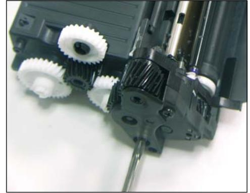
44. Install the gearside end plate as shown.
