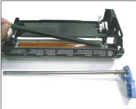
21. Remove the PCR and clean with a damp cloth. Allow it to dry before installing.
