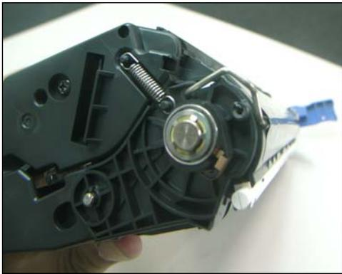
54. Install the tension spring that was removed in steps 10 and 11.
