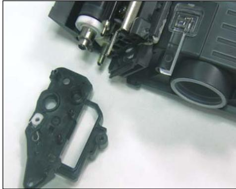
28. Roller support plate removed.
