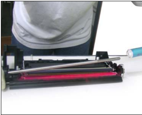
56 Slide out the drum as shown.
