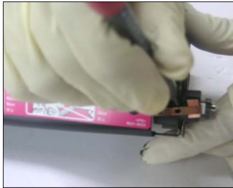
48 Insert a small flat screwdriver into a small hole located under the contact. Tilt the screwdriver to push it out.
