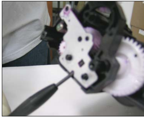
16 Remove the metal plate by prying it off with a small flat screwdriver.
