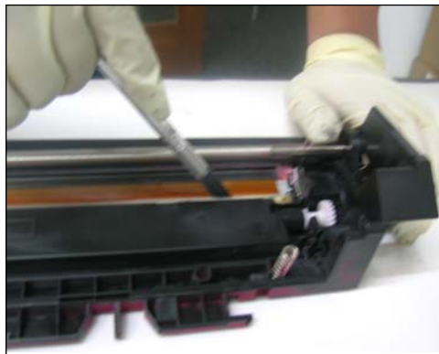
59 To remove the wiper blade, cut the factory adhesive so it allows you to remove the blade.
