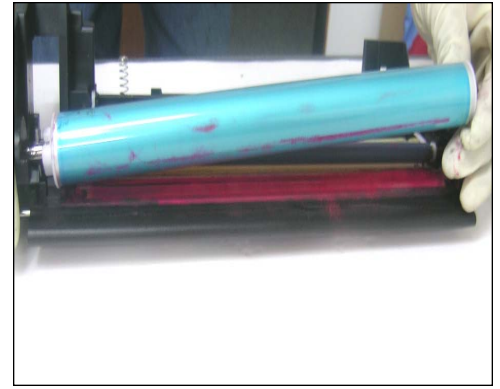
55 Tilt the drum and axle at a 30-degree angle to remove the drum.
