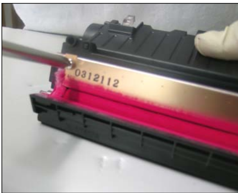
27 Remove the doctor blade by first removing the left and right screws as shown.
