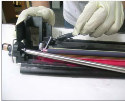
57 Remove the PCR roller by unclipping both sides as shown.
