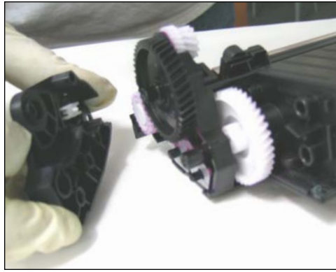
13 Pull the end-cap off to expose the outer gears.
