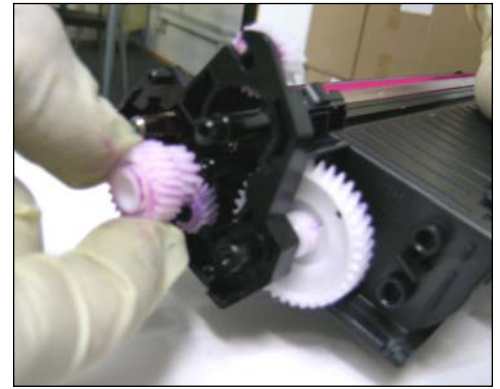
17 Remove first inner-gear as shown.
