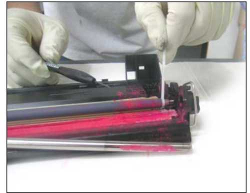
57 Remove the PCR roller by unclipping both sides as shown.
