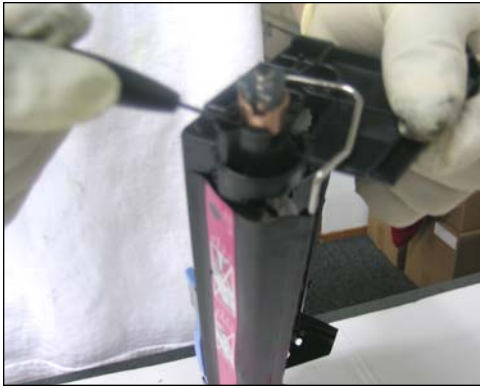
53 Pry out the axle bearing as shown.
