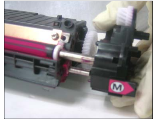
23 The roller support should slide out very easily.
