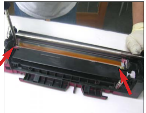
60 Remove the wiper blade by unscrewing both sides as shown.
