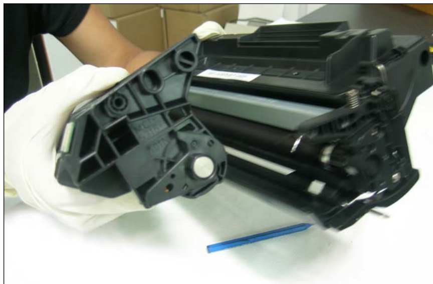
35. Holding the drum shutter open, join the toner hopper and waste hopper.
