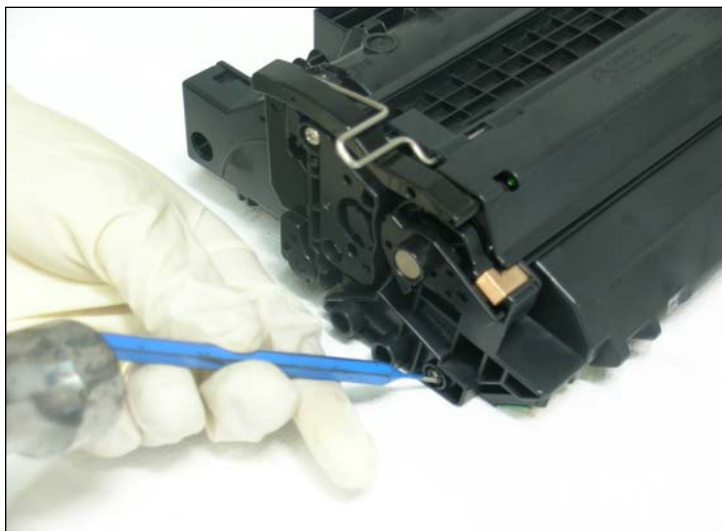
36. Install the cartridge pins into each end of the cartridge. Test the cartridge.
