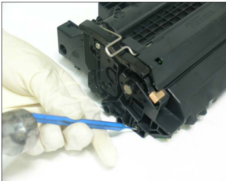
2. Using a small drift-punch and a hammer, carefully tap the cartridge pins into the waste hopper.
