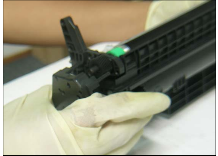
20. Slide the gear housing end cap away from the toner hopper.
