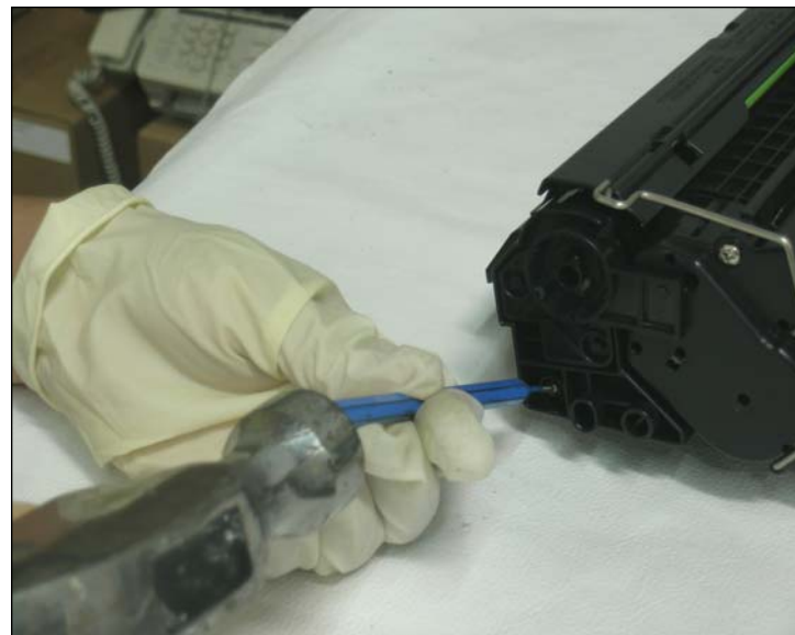
2. Using a small drift-punch and a hammer, carefully tap the cartridge pins into the waste hopper.
