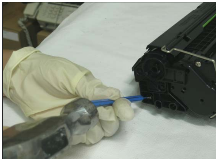
36. Install the cartridge pins into each end of the cartridge. Test the cartridge.
