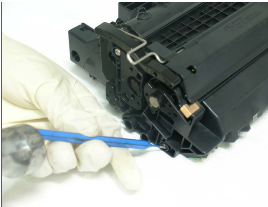
1. Place the cartridge on the workbench so the drum faces up.
