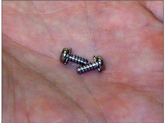
12. On the toner supply chamber right side, remove the two screws and end cap. Note that these screws have lock washers.
