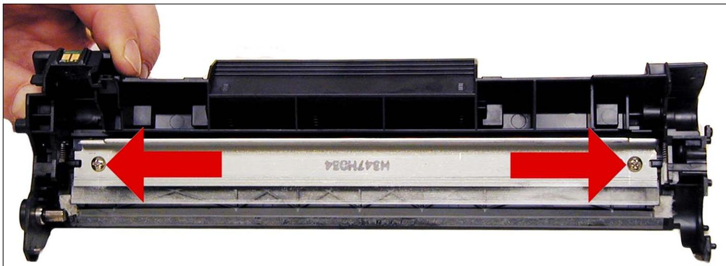
6. Remove the two screws and the wiper blade.
