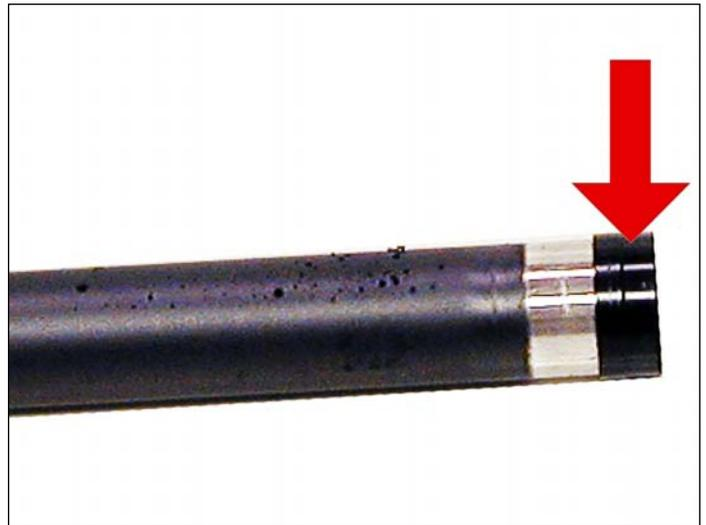
15. Remove the magnetic roller assembly. Be careful of the bushings! They are very fragile.
