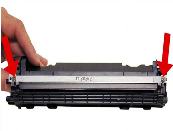
16. Remove the doctor blade and two screws.
