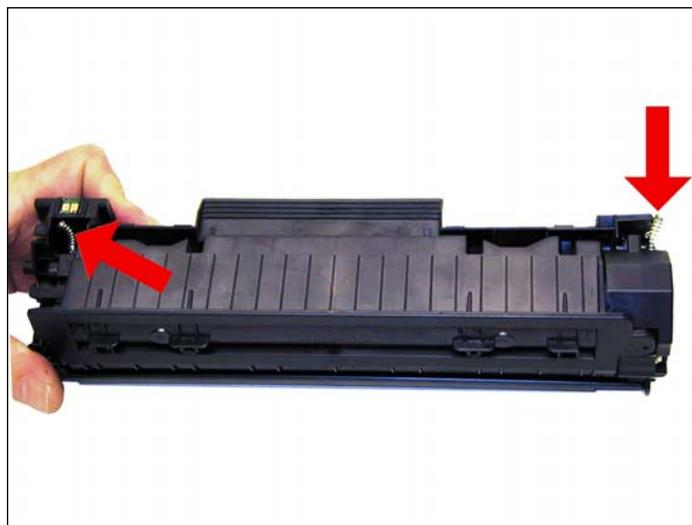
2. With a pair of needle nose pliers, release both the hopper tension springs.
