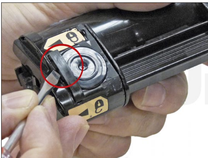
6. Pry up the chip cover, and then the chip from the end cap and replace.
