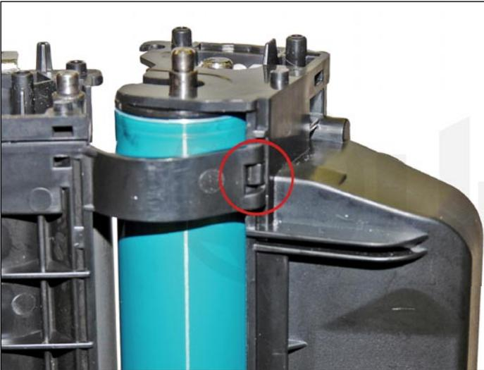
32. Place the two halves together by setting the curved bottom clips into the toner hopper.
