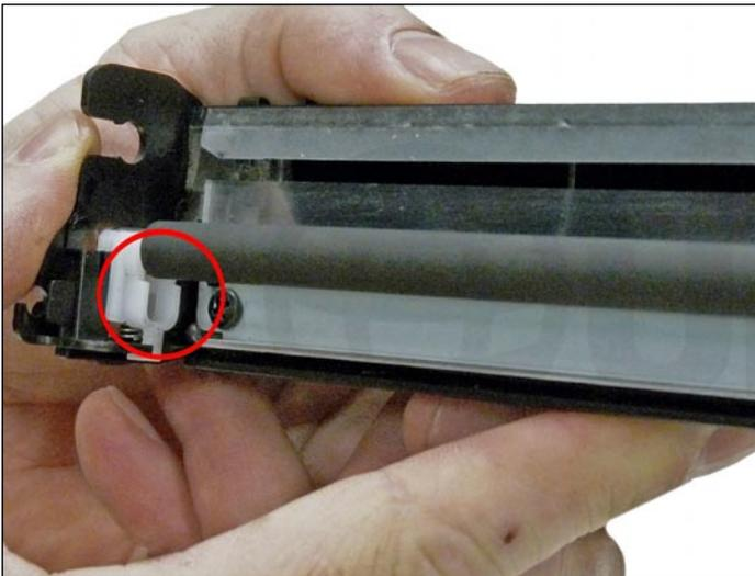
19. Place a small amount of conductive grease in the holders, and install the PCR.
