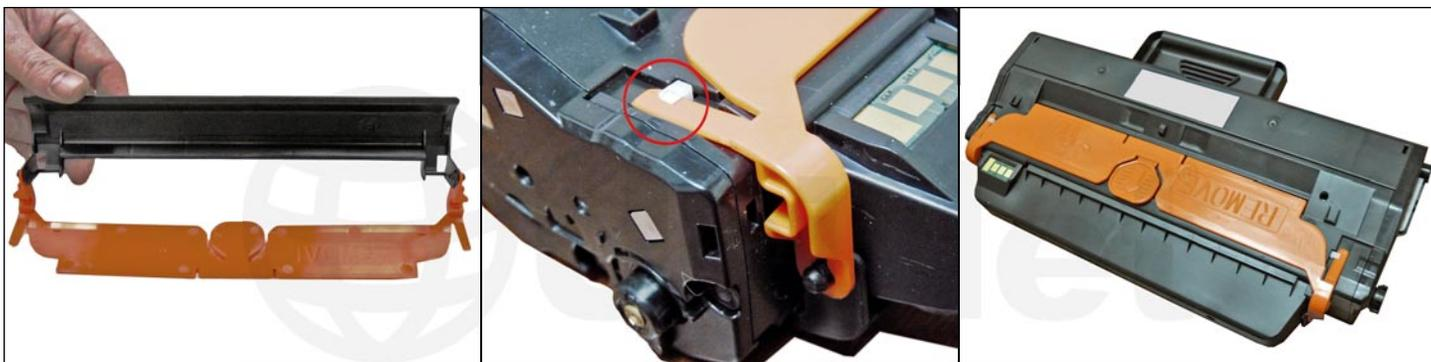
39. Install the drum cover assembly by sliding the bottom black part of the drum cover over the drum, and sliding the orange top part so that the two small tabs on each side fit under the white locking tabs located on each side of the cartridge.
