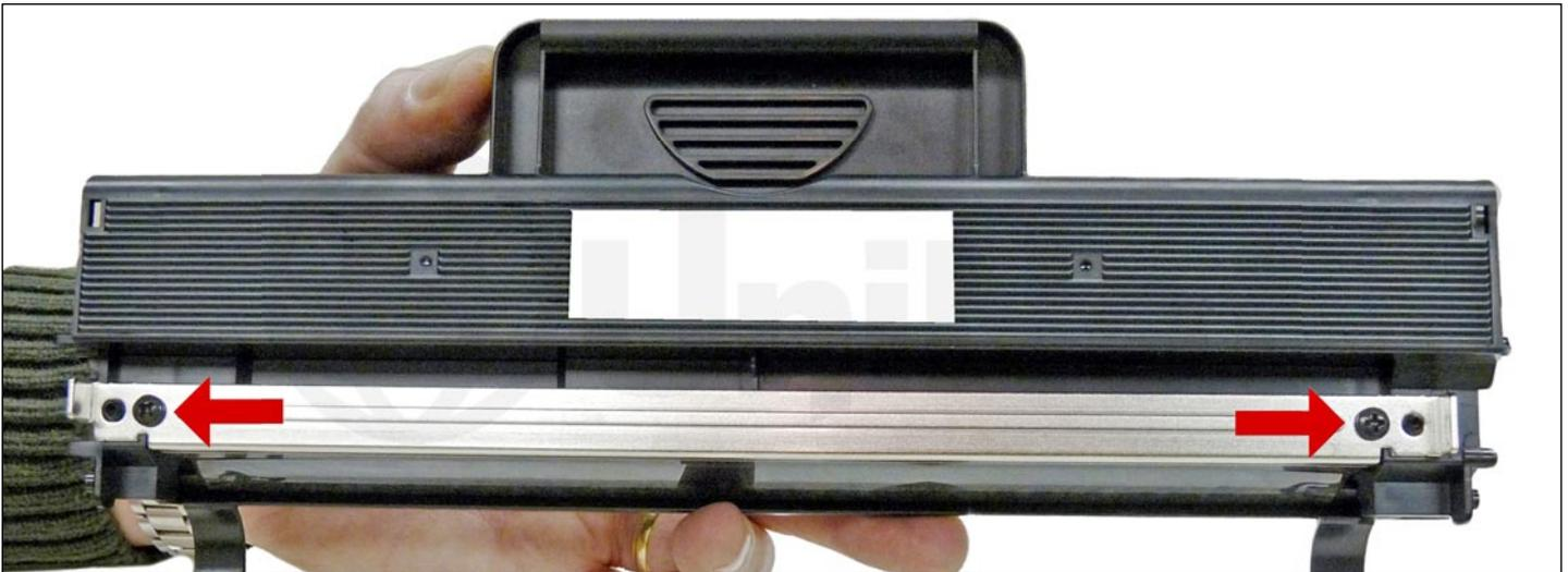
28. Install the doctor blade and two screws.
