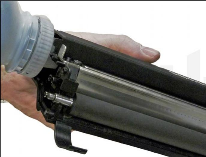
30. Fill the hopper with toner for use in the Dell B1260 series, replace the fill plug, and check for leaks.
