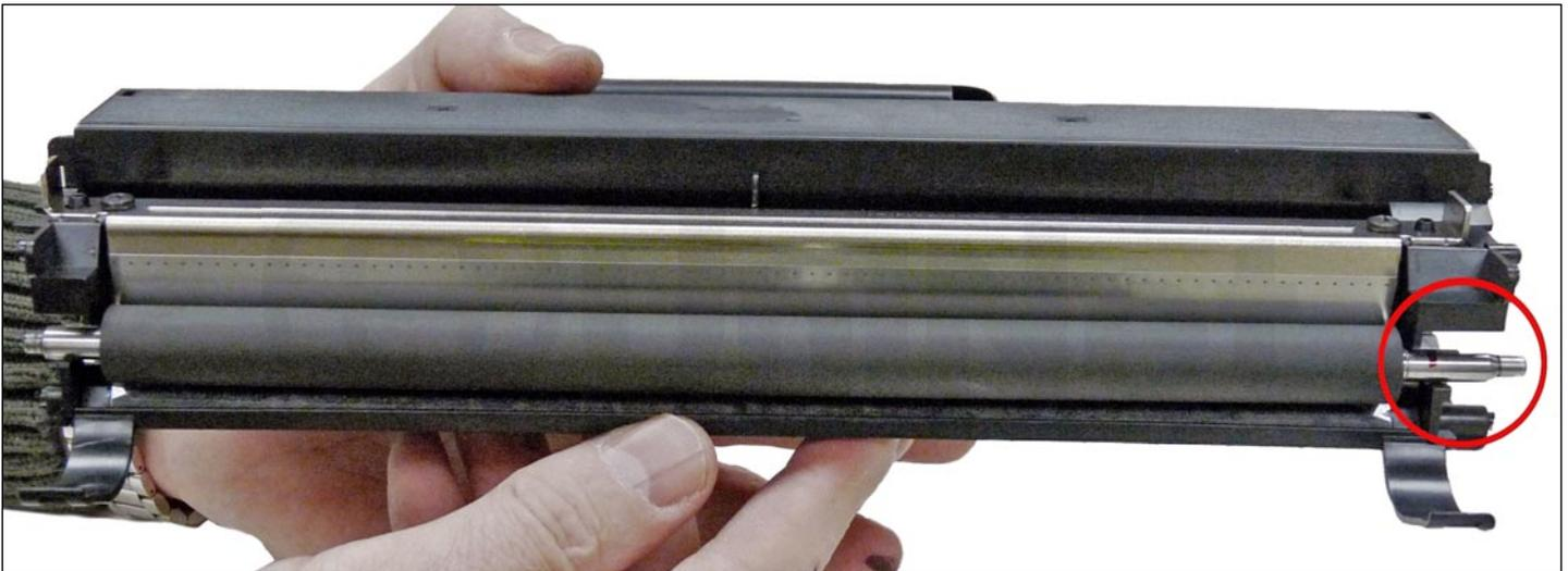
29. Clean the developer roller with a dedicated developer roller cleaner and replace into the hopper.
