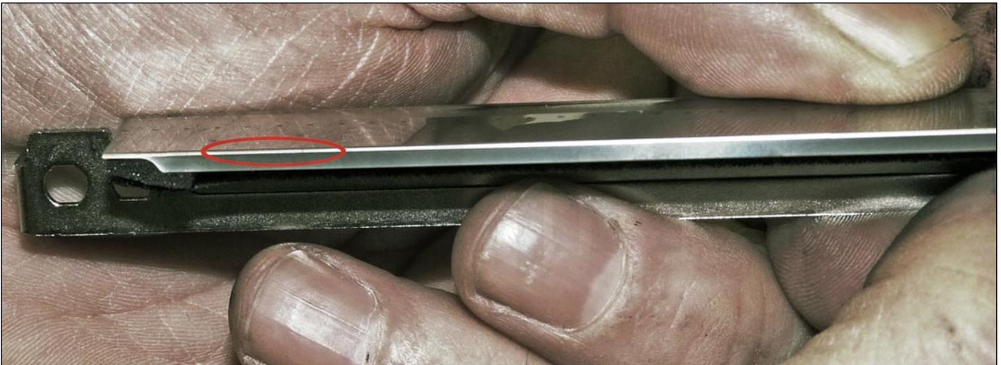
27. Clean the doctor blade's edge so there is no evidence of build up along the edge. If any buildup exists, the cartridge will streak. No chemicals should be used. We have found using a clean ice cream-type wooden stick works great for scraping the blade clean without damaging it.
