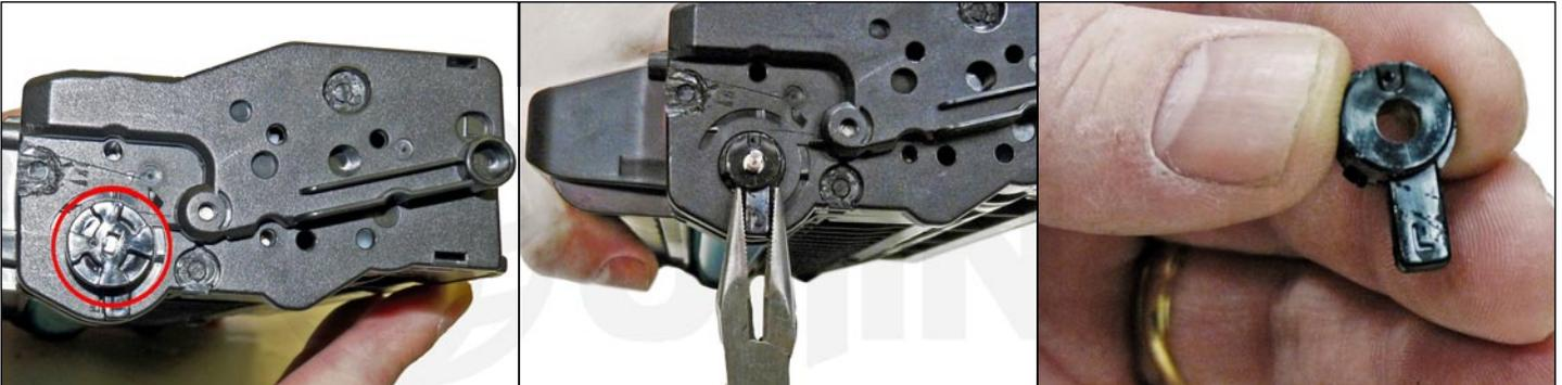
5. On the drum-gear end cap, remove the drum-drive gear and the remaining arm the same way as the right side. Turn it to be straight down, and pull it straight out. Press in on the top tab and bottom tabs and remove the end cap. Note that the arm is stamped with the letter **L**.
