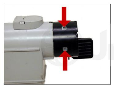
1. Carefully pry off the colored end cap by lifting up on the plastic around the tabs.
