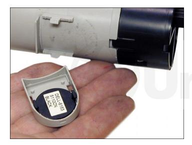
7. Separate the chip from the holder and replace the chip.
