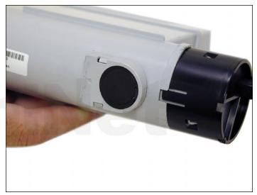
8. Snap the chip holder back on the cartridge.
