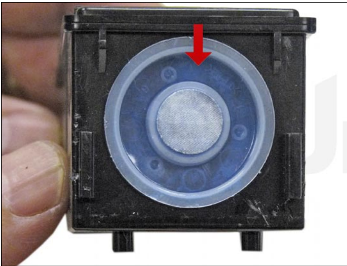
4. Remove the fill plug and clean out all remaining toner.
