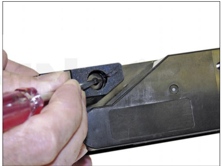
5. Press in on the waste toner port and vacuum all the waste toner out from the cartridge.
