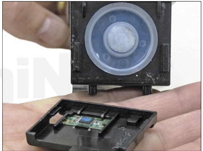
3. Pry up the two tabs on the end cap and remove.
