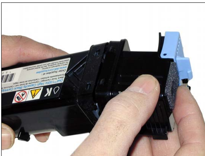
9. Install the waste chamber on to the supply hopper.
