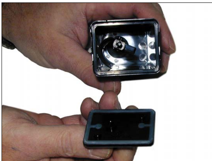
4. Remove the supply hopper cover. Clean out any remaining toner.
