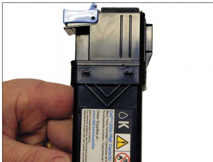
10. Make sure all four tabs are locked in place.
