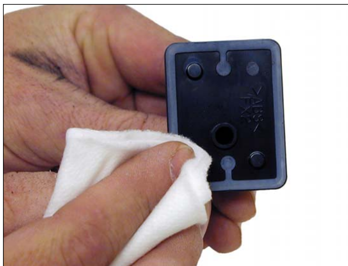
5. With a clean lint free cloth, wipe down the seals on both sides of the cover. No chemicals are needed to clean it, just the cloth.
