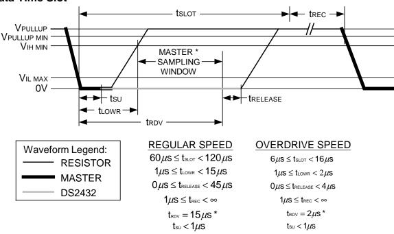
\*The optimal sampling point for the master is as close as possible to the end time of the  $t_{RDV}$  period without exceeding  $t_{RDV}$ . For the case of a Read-one time slot, this maximizes the amount of time for the pull-up resistor to recover the line to a high level. For a Read-zero time slot it ensures that a read will occur before the fastest 1-Wire device releases the line ( $t_{RELEASE} = 0$ ).
