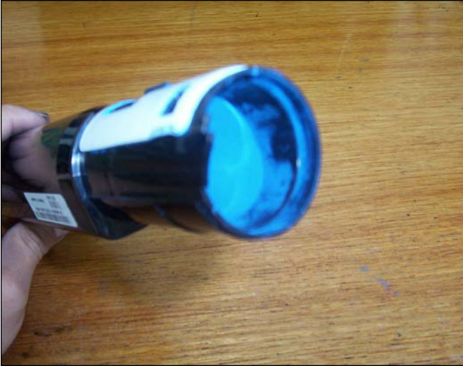
7. This is the carrier chamber, empty it out and you will find the toner fill plug. Remove it to clean cartridge and fill toner.
