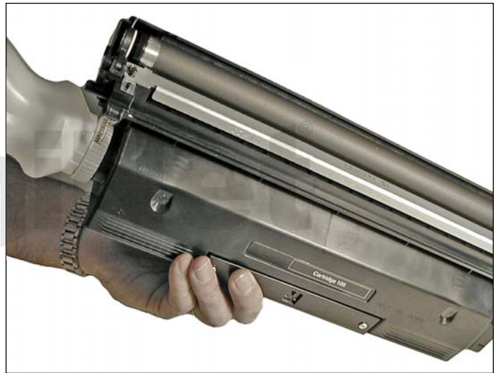
30. Fill the toner hopper with 500 grams of toner for use in the Canon EP 105 cartridge. Replace the fill plug.
