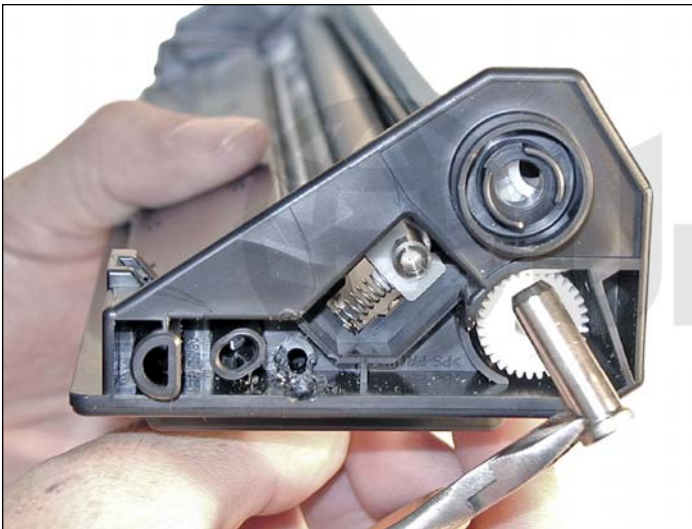
4. On the small gear side, remove the metal axle pin with wire cutters. The pin comes out easily, and there are already two notches in the plastic that allow the wire cutters access.
