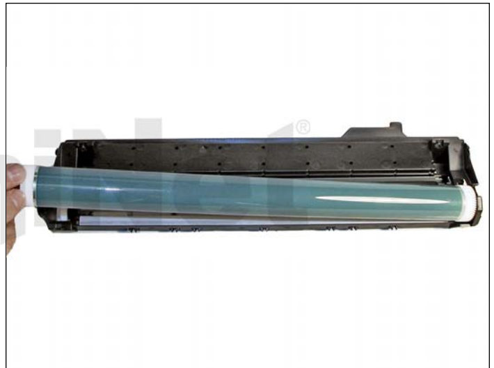
5. Remove the photoconductive drum, and place aside.
