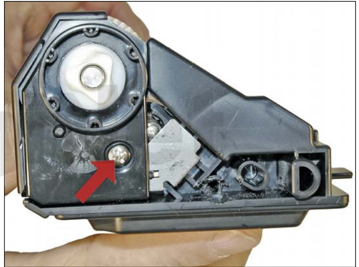
3. On the large gear side, remove the drum alignment plate and screw.
