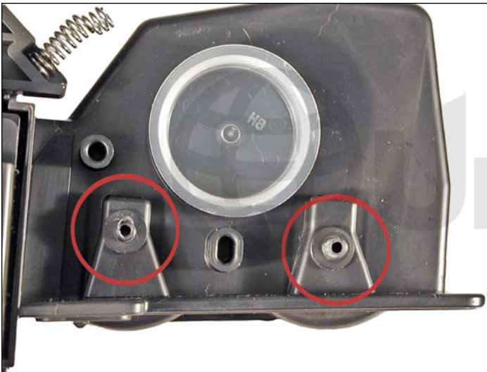
31. While holding the remaining end cap in place, drill two small shallow holes into where the plastic pins once were.
