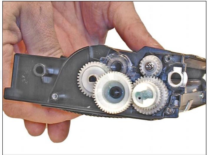
12. Clean the gears, making sure that they have no toner on them. This is a good time to also check the gear shafts to make sure there is enough grease. If the shafts appear dry, or the grease is contaminated with toner, clean the shaft and inside of the gear. Replace the grease with white lithium grease.
