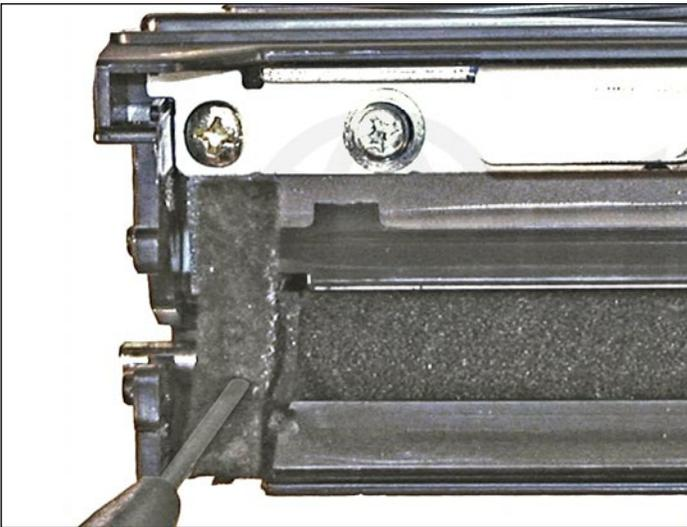
11. Inspect the magnetic roller felts. If they are compressed (shiny), roughen them up with a small screwdriver.
