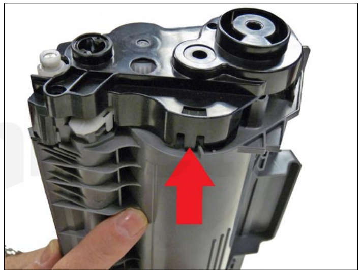
3. Press in on the bottom tab and remove the end cap.
