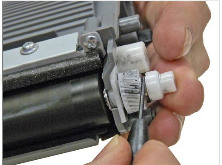
5. Remove the white plastic spacer from the developer roller shaft.
