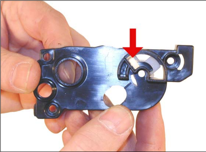
17. Set the flag gear, install the gear cover plate, and three screws.
