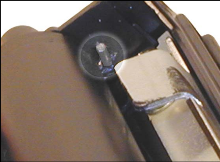
4. Locate the two tabs on the developer roller end plate and pry off.
