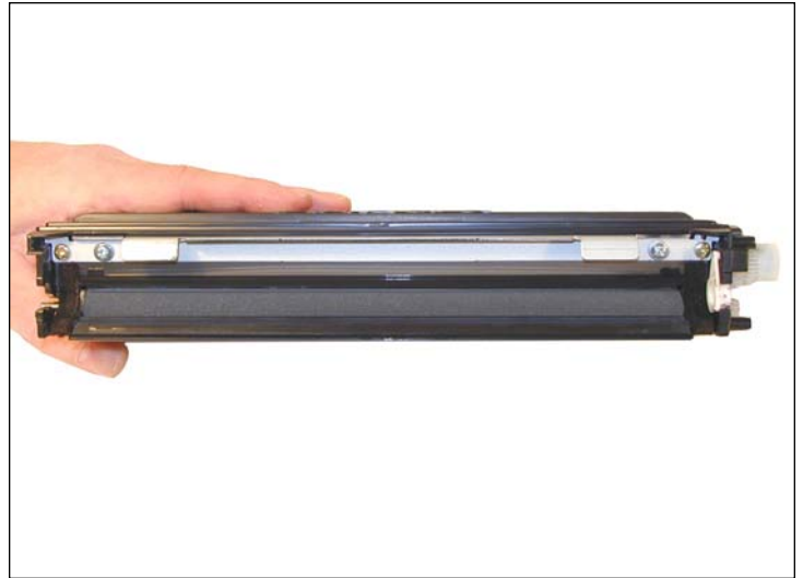
10. Vacuum the doctor blade and foam feed roller clean. We do not recommend that the doctor blade be removed and the developer roller felt seals will be disturbed. Once a new blade is available, great care will have to be taken not to tear the seals, causing a leak. The doctor blade can be easily cleaned by blowing the excess toner off, and wiping down with a lint free cloth. Be very careful not to leave any lint behind!
