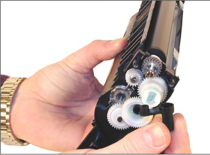
7. Remove the black plastic spacer from the developer roller shaft.
