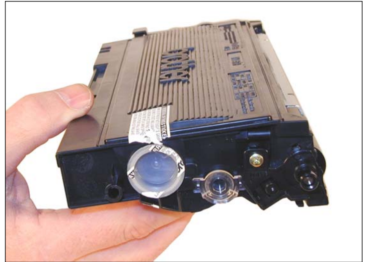
19. Replace the fill plug. Wipe the cartridge down to remove any remaining toner dust.
