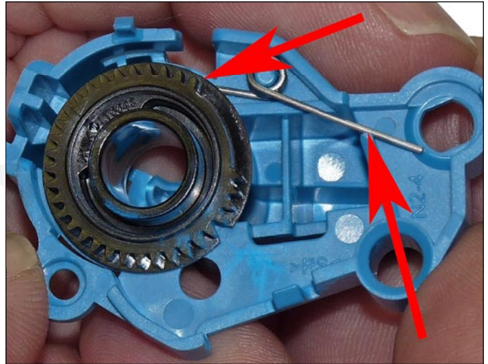
27. Set the gear and spring as shown. This is the proper reset gear position. The gear and spring must be set EXACTLY as shown. If you have a starter cartridge, these gears will not be present. Aftermarket gear and spring sets are available for both cartridges.
