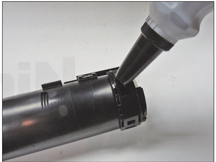
5. Fill with toner for use in the Phaser 3610.
