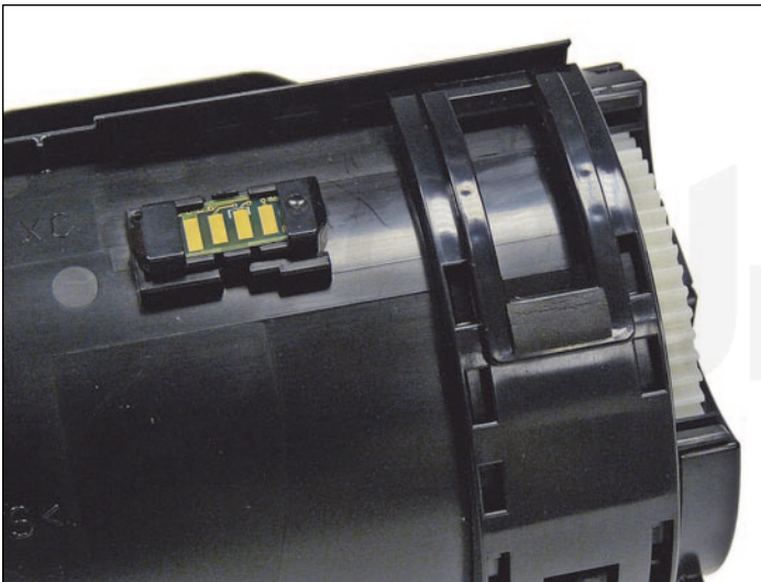
6. Slide the toner port cover back in place.
